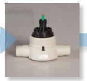
6 Put inner housing into body. The inner housing must fall into place. If you need to push the housing in, there is a misalignment
