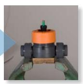
8 Hand tighten the housing nut as far as you can.
