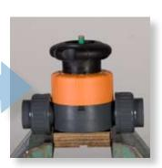
1 2 Attach the handwheel to the spindle. Don't apply force, just turn it slightly until it falls onto the spindle There should be a "klick"
