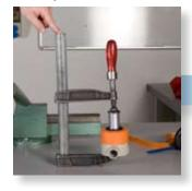
Use a C-clamp to pretension the inner housing. Tighten the housing nut to the dedicated position
