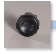
Screw in the diaphragin. handlight clockwise into Screw in the diaphragm. the inner housing and then turn it back min 90°. Turn the spindle into open position while holding the diaphragm in place. The diaphragm tabs must be positioned between the guiding bars of the inner housing.
