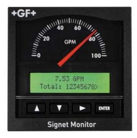
The Signet 5075 Totalizing Flow Monitor features a traditional analog dial for flow rate at a glance while the backlit LCD provides precision flow rate, total volume and programming information.
