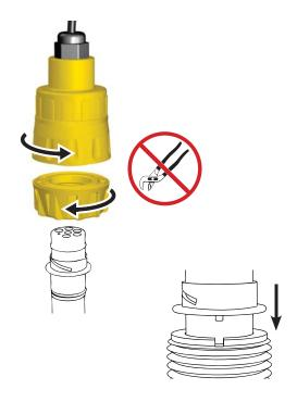
Do Not Use Lubricant or Sealing Tape on Threads. Do Not Overtighten.
