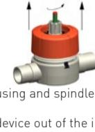
8. Take inner housing and spindle assembly out of the valve body
