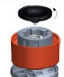
5. Hold hand wheel tight. Screw new diaphragm handtight clockwise into the inner housing and then turn the diaphragm back by min. 90°.
