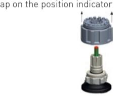
9. Push spindle device out of the inner housing with a little tap on the position indicator
