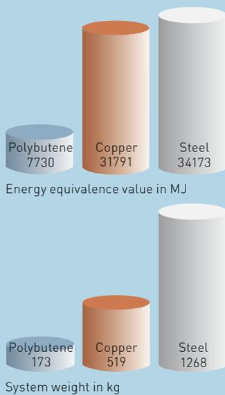
Another advantage of plastic is its low weight. This makes it significantly easier to handle and transport components. Unlike a metal system, you won't need a crane to install a plastic system.
