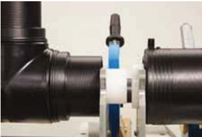
Socket fusion in a fusion machine
