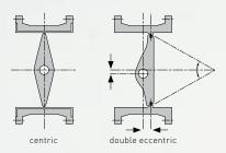
Butterfly valves are normally built according to a centric operating principle. The new butterfly valve from GF Piping Systems, however, works on a double eccentric operating principle. The result of this principle is that the disc does not come into contact with the seal when in the open position, thus warranting good friction behavior and less wear and tear. Thanks to double eccentricity, protection against water hammer is improved as well.
