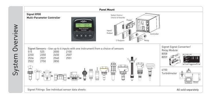
There are hundreds of system types that can be set up with the 8900. The examples below illustrate various sensors in different installation schemes. Wiring topology for point-to-point, daisy-chain, multi-drop, or a combination of these are listed in each example. Digital sensor outputs allow for long cable runs with high noise immunity. See Wiring section for allowable cable lengths.
