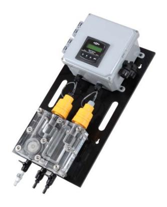
The Signet 4630 Chlorine Analyzer System is an integrated all-in-one system designed to measure free chlorine. The 3-4630-21 chlorine panel with the optional pH sensor is used to accurately calculate free chlorine in applications that have varying pH values (±0.20 pH units).
